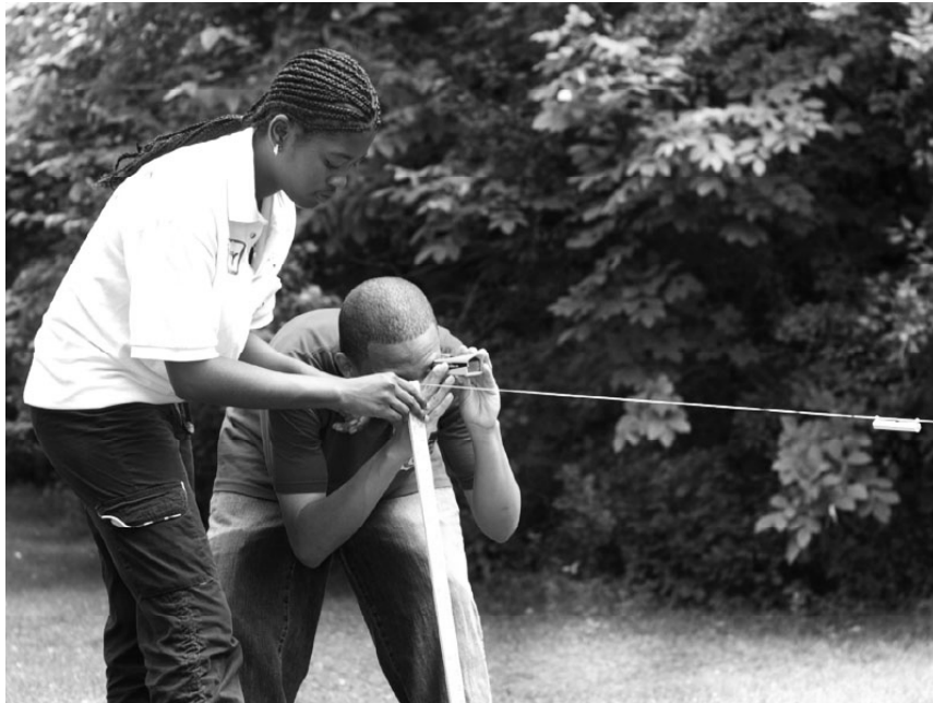
One student adjusts the meter stick to be vertical, while another uses the scope level to spot a point uphill.
